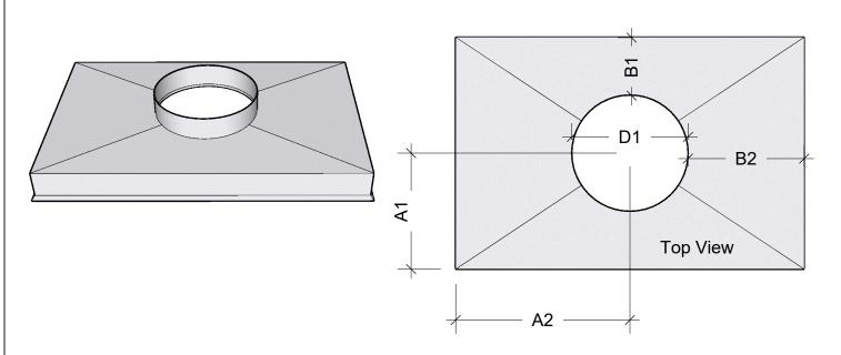
Flue dimensions may be provided by measuring to the center of the flue (A1 and A2) and specifying the hole diameter (D1), or by measuring to the side of the flue (B1 and B2) along with dimension D1.
