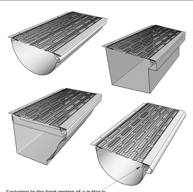
Fastening to the front portion of a gutter is recommended but optional for all gutter profiles where the front edge of the gutter screen hooks into place like a hanger. On Euro bead gutters, the profile does not allow for a hook, therefore fastening is strongly recommended.
