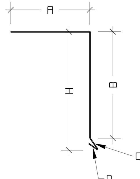
Available in 0.027" aluminum, Kynar 0.032" aluminum and 24 gauge steel, 24 gauge galvalume, copper, freedom gray, lead coated copper and 24 gauge stainless steel.
