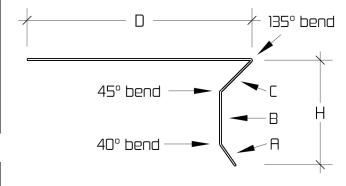
Available in 0.027" aluminum, Kynar™ 0.032" aluminum and 24 gauge steel, 24 gauge galvalume, copper, freedom gray, lead coated copper and 24 gauge stainless steel.
