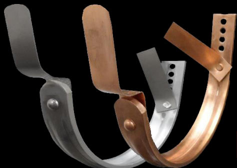
#15 Pressed Formed Hanger 3/16" Bar Stock with Stiffening Wedge 5", 6", 8" Fascia Mount
